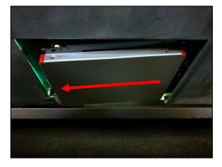
Once the SSD has been removed, you will need to take the plastic bracket from it, and fit this to the new SSD, as pictured below. This is stuck in place with tape, so can be pulled off carefully. Ensure the screw holes on the bracket line up with those on the SSD.
