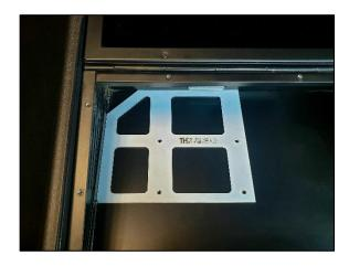
Once space has been cleared, the drill guide can be placed in top left corner of the chassis base. See the picture to the left. Note the orientation of the guide and ensure the text "this side up" is facing up. Also ensure the guide is right in the corner and flush with both edges of the chassis.
