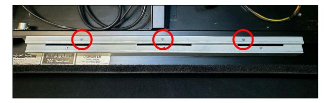
Once the support bracket is screwed in place, the arm rest can then be fitted. To attach this correctly, follow the three images below. The arm rest should first be placed in roughly at a 45-degree angle, before being placed down, and finally pulled towards the front of the console as much as possible, using a little force.
