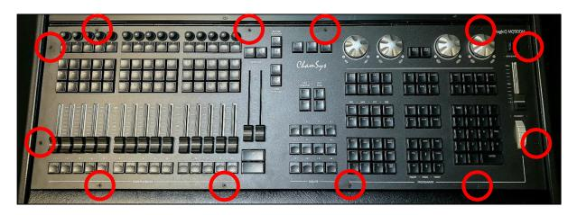
Once all these steps have been completed, the upgrade process is finished and you will have an MQ500M spec console with the new front panel fitted, as pictured below. We now recommend switching the console on and fully testing the new front panel, ensuring all motorised faders, keys, encoders etc are all working correctly.
