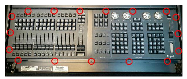
Once all 17 screws have been removed, the front panel assembly can then be lifted carefully from the front. Note that the assembly consists of 2 front panels, and each panel has a cable that must be disconnected to free the assembly completely, as pictured below. Both are locking connectors; push the tab to unlock and pull to release. Once these are disconnected, remove the front panel assembly, and set aside.
