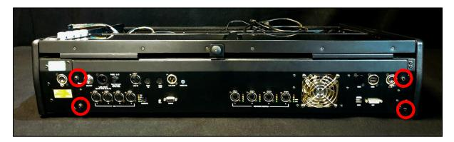
To begin, turn the console around to access the rear and remove the 4x M4 hex screws securing the rear panel in place, using a 4mm ball driver or Allen key. See the image above for screw locations. Once these screws are removed, you can carefully slide the rear panel out, just enough so all components can be accessed as in the image below.
