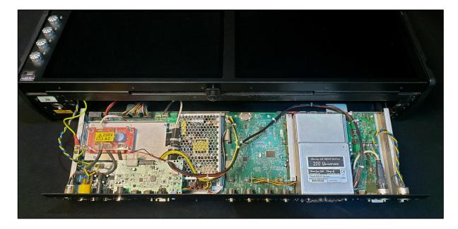
With the rear panel pulled out, you can now easily reconnect the 2x display port connectors and audio jack, as pictured to the right. Feed these back through the hole from the chassis. Ensure the display port connectors are in the correct ports, as marked earlier.
