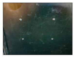
Screw through the bottom of the chassis into the power supply. See the images on the next page of the 4 screw holes to be used on the power supply, and correct orientation.
