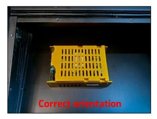
Finally, connect both cables to the power supply. See the first image below for the correct orientation of each cable. The AC card cable should then be fed through the hole in the middle of the chassis, over into the rear panel, pictured in the second image below.
