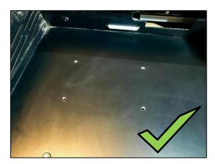
Once the area is clean, lift the console from the front and file out the holes from the underside so they are smooth, and screws will comfortably fit through.
