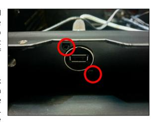
**Option 2:** Using some force, pull the white cable away from the USB socket. This will likely break the socket, but this is no longer required. You may also need to cut the heat shrink away first if it will not come away.
