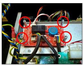
Once all connections have been removed, the AC card can now be removed by unscrewing the 4x M3x12 spacers, as highlighted in the picture above, right, using a 5.5mm nut spinner or spanner. The old AC card can then be removed, and the new AC card fitted in its place with the same orientation, replacing the 4x M3x12 spacers.
