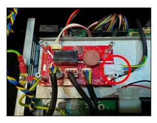
When you have secured the new AC card in place with the 4x spacers, now replace all 4x connections previously removed. See the picture to the left for locations and orientations for these.
